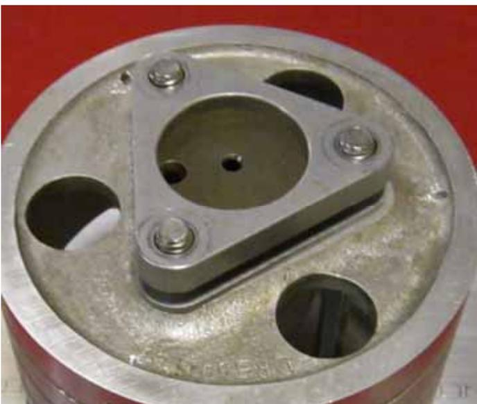
Fig 3 Slip Driver-Capture Plate over bolts as shown
