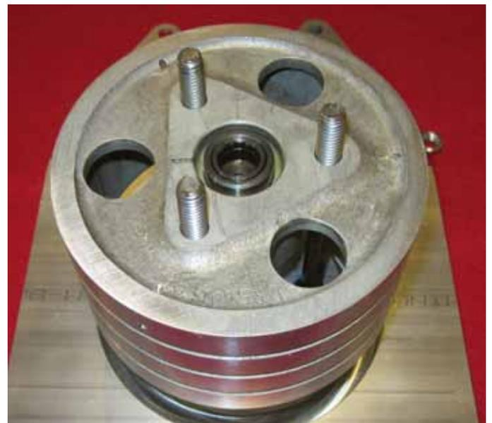
Fig 4 Lifter seated on internal lock ring in Dashpot as shown
