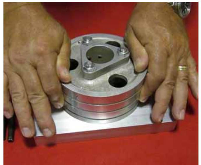
Fig 4 Verify that all air is removed from Hydraulic unit. If it is properly filled and bled, it will feel like it is stuck or locked up.
