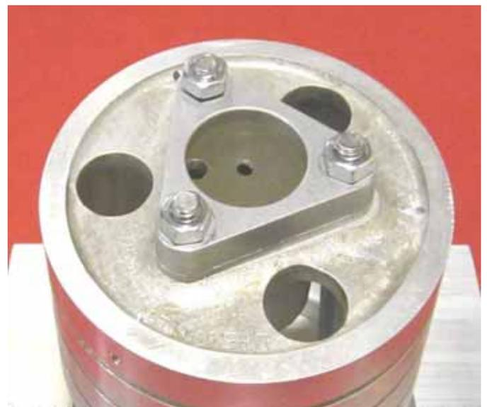
Fig 4 Screw lock-nuts on bolts (deformed thread UP) as shown
