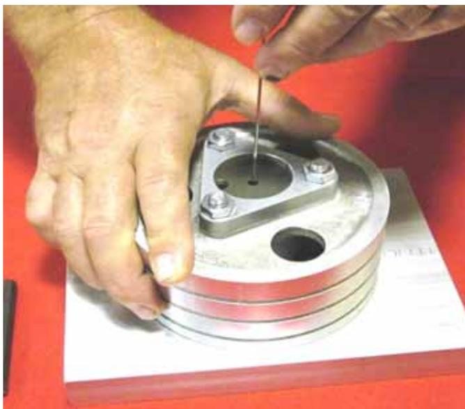
Fig 3 Insert clean bleed-wire into center hole to open ball check in the lifter unit below.
